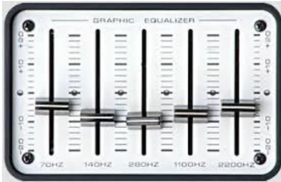
Figure 6 A 5-band graphic equalizer. Each slider represents the power/intensity of sound at the various frequencies (ranging from 70Hz on the left to 2200 Hz) on the right. The current settings here have a slight emphasis on the low and high end, with a dip in t
